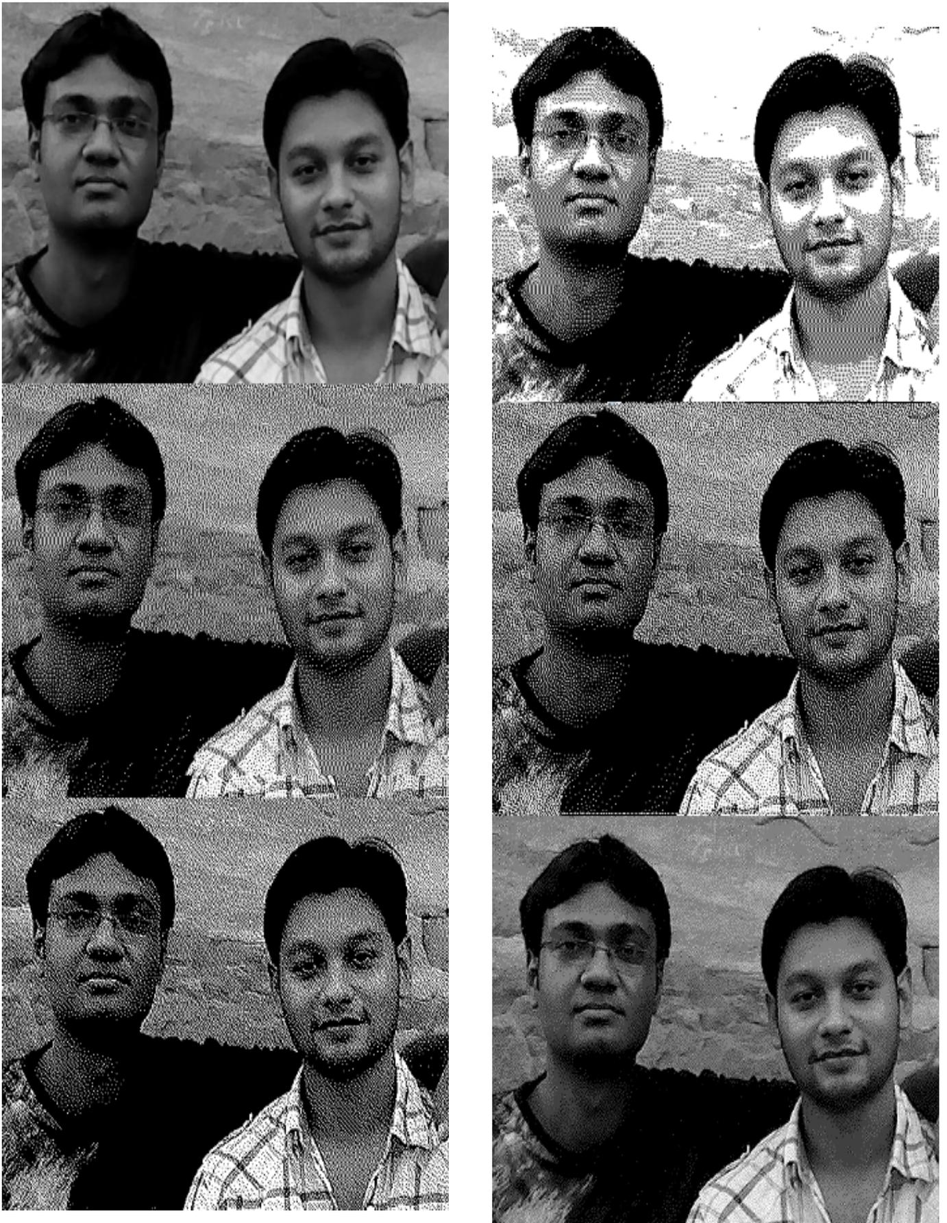
Figure 8: (Original image, Error Diffusion, Floyd's technique[4], Jarvis's Technique[3], AI, TAIH-in that order from left to right, top to bottom)
