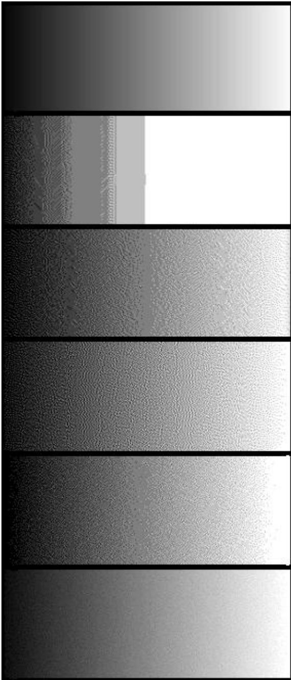
Figure 9: REPRODUCTION OF GRAYSCALE RANGE (Original image, Error Diffusion, Floyd's technique, Jarvis's Technique, AI, TAIH-in that order from top to bottom)
